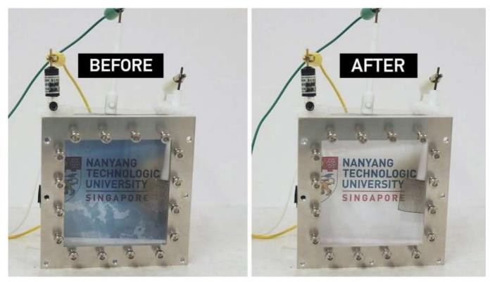
The new energy-saving material for electrochromic (EC) windows blocks ray without compromising views through the window, as it allows up to 90 per cent of visible light to pass through. Credit: Nanyang Technological University
